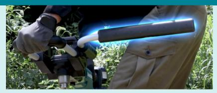
Earth auger attachment and side bar provides added control and reduces kickback
